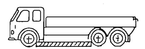
4.5.2. "Ground clearance beneath one axle" means the distance beneath the highest point of the arc of a circle passing through the centre of the tyre footprint of the wheels on one axle (the inner wheels in the case of twin tyres) and touching the lowest fixed point of the vehicle between the wheels.
