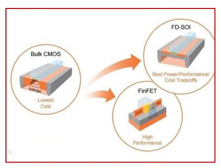
A major target in chip design and fabrication is to reduce and control the current - which activates the transistor gate<sup>5</sup> - and accordingly, the performance of the chip (switching speed & power consumption).
