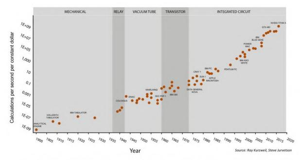
One famous representation of the processor industry is Moore's Law. This describes how the number of transistors in a chip doubles roughly every 18 months. This was true for a very long time, but is starting to slow down. Transistors are getting so small that we are nearing the limit of what physics will allow.
