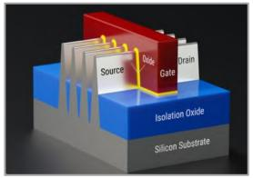
Chips utilizing FinFET have been on the market since the first half of the 2010s with Intel commercializing 22nm FinFET in 2011. With continuous optimization of the transistor density per chip, it has become the dominant design at 14nm, 10nm, 7nm and 5nm process nodes. The state of the art in FinFET is nominally 5 nm today, produced by TSMC and Samsung, with 3 nm in pre-production. Although European companies design in FinFET, they rely on foundries such as TSMC and Samsung for
