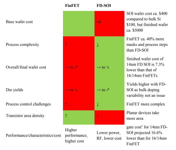
However, FD- SOI is well suited to achieving a **better performance** / **power consumption trade-off at functionally equivalent nodes.**<sup>8</sup> It is fair to say that the two technologies compete in many applications including automotive, AI, IoT, 5G/6G, and industrial manufacturing.
