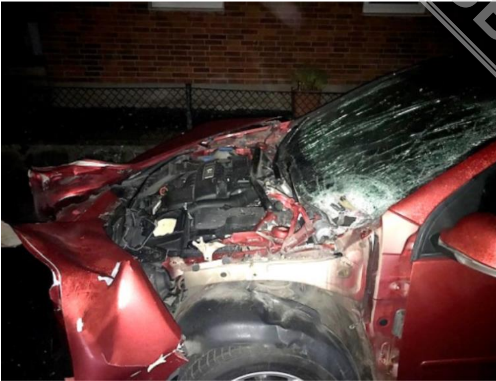
The effect of one flash banger with a pyrotechnic composition of 80-100 g NEC after being detonated outside of a car, near the front window. The impact has torn the hood away completely. Photo: Swedish Police Authority
