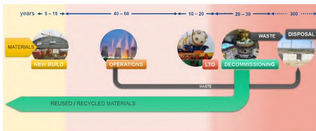
Figure 20 – Nuclear installation life-cycle
