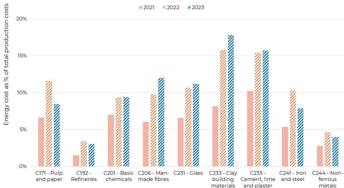
Figure 15: Estimated energy costs (as shares of production costs) for manufacturing sectors in 2021–2023, EU average
