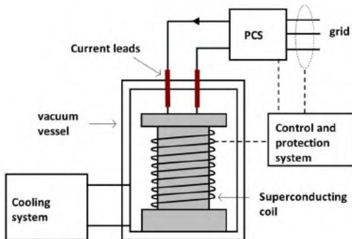
This technology is characterized by high power density. Hence, it would be prone to provide power systems with fast services. SMES are considered to be still under development; many researchers are investigating the potential of this kind of storage. Costs are currently high and extremely volatile, ranging from 300 to 2000 €/kWh [54], but are expected to fall to around 200 €/kWh by 2050 [40].
