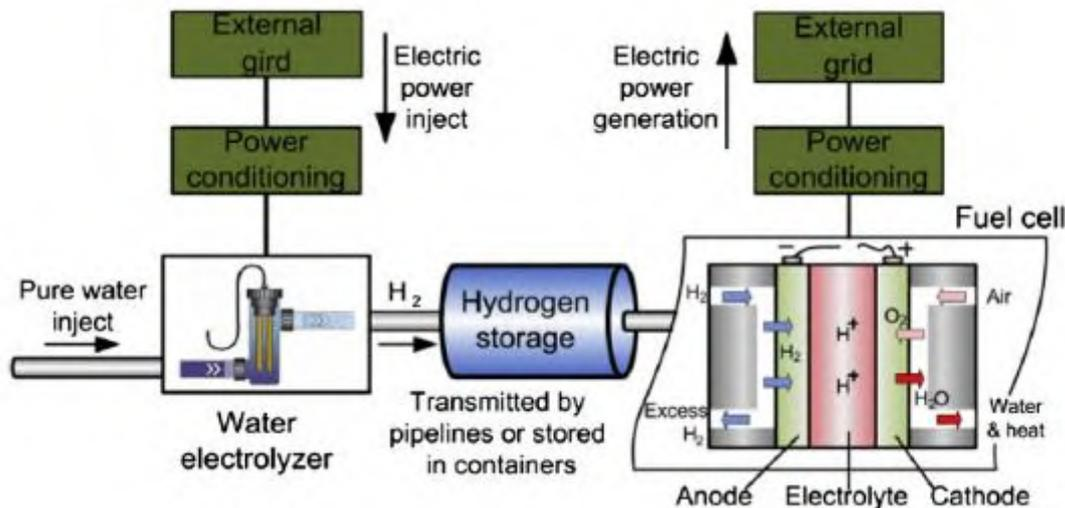
Despite the low efficiency, which hardly exceeds 45 %, this technology has gained great attention because of the high density of energy, of the capacity to store for long periods and the suitability for large scale storage [32]; in a scenario of high penetration of renewables, P2H is expected to have a prominent role providing a cost-effective storage solution [56].. Costs are likely to decrease by more than 30 % by 2025 [55].
