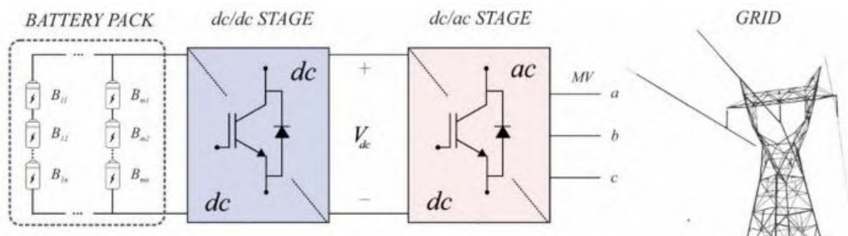
This kind of storage has the advantage of being highly modular, cells can be connected in different configurations in order to reach the desired voltage, energy capacity and power, but care must be taken to prevent non-optimal usage from rapidly reducing battery life or even damaging it. The technology is currently increasing its market penetration, exploiting the significant progress made in terms of cost and lifecycle.
