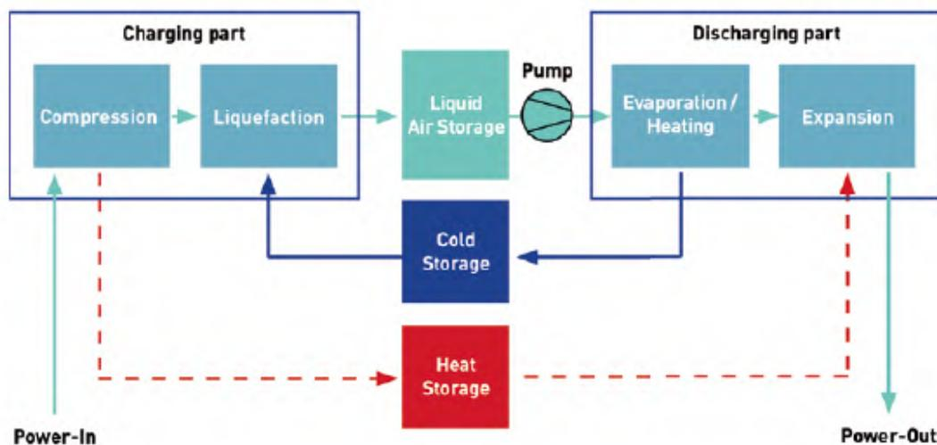
The advantage of LAES over CAES is that it does not come with any geographical restriction, as the high energy density allows the use of tanks to store the liquified air [39]. The cost of the technology is 250÷600 €/kWh and is expected to decrease to 150÷400 €/kWh by 2030 [40].
