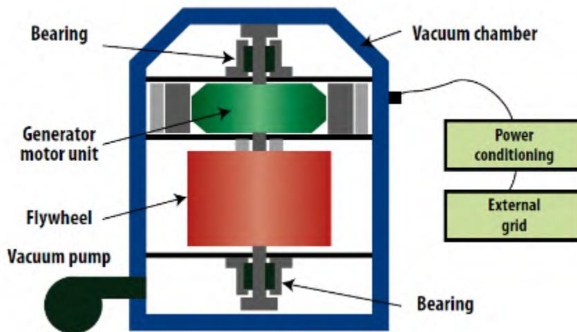
There are two types of flywheel: low-speed (<10000 rpm) and high-speed (up to 100000 rpm). The former is made of metallic materials, is easier to build and is characterized by higher weights; hence, it is more suitable for stationary applications. The latter is made of composite materials, such as carbon fibres, which provide better performances at higher costs; this option is adopted for low-energy applications [25], [40].
