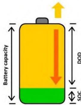
Their roundtrip efficiency is in the range 70÷90 % and their cost is around 120÷200€/kWh. These two characteristics make lead-acid batteries one of the most convenient batteries in terms of performance/cost trade-off. Limited improvements in the manufacturing process are expected, which may lead to reduce the cost below 100€/kWh while maintaining similar RTE [27], [40].
