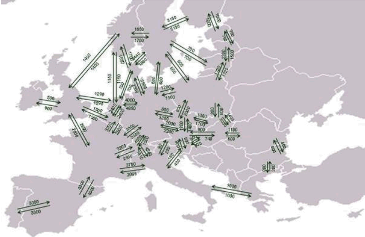
Map 6: Interconnection capacity requirements 2020 in MW 47 , PRIMES Reference scenario (source: KEMA, Imperial College London)
