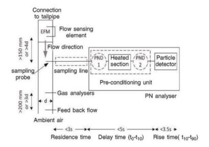
The PN analyser shall be connected to the sampling point via a sampling probe which extracts a sample from the centreline of the tailpipe tube. As specified in paragraph 3.5. of Appendix 4, if particles are not diluted at the tailpipe, the sampling line shall be heated to a minimum temperature of 373 K (100 °C) until the point of first dilution of the PN analyser or the particle detector of the analyser. The residence time in the sampling line shall be less than 3 s.
