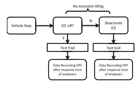
2.6.7. "Validation of PEMS" means the process of evaluating on a chassis dynamometer the correct installation and functionality within the given accuracy limits of a Portable Emissions Measurement System and exhaust mass flow rate measurements as obtained from one or multiple non-traceable exhaust mass flow meters or as calculated from sensors or ECU signals.
