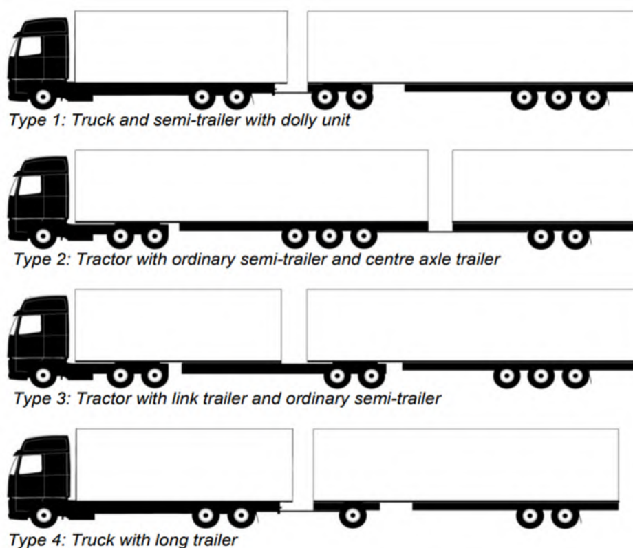
Figure 4: Typical EMS combinations used in European freight transport.
