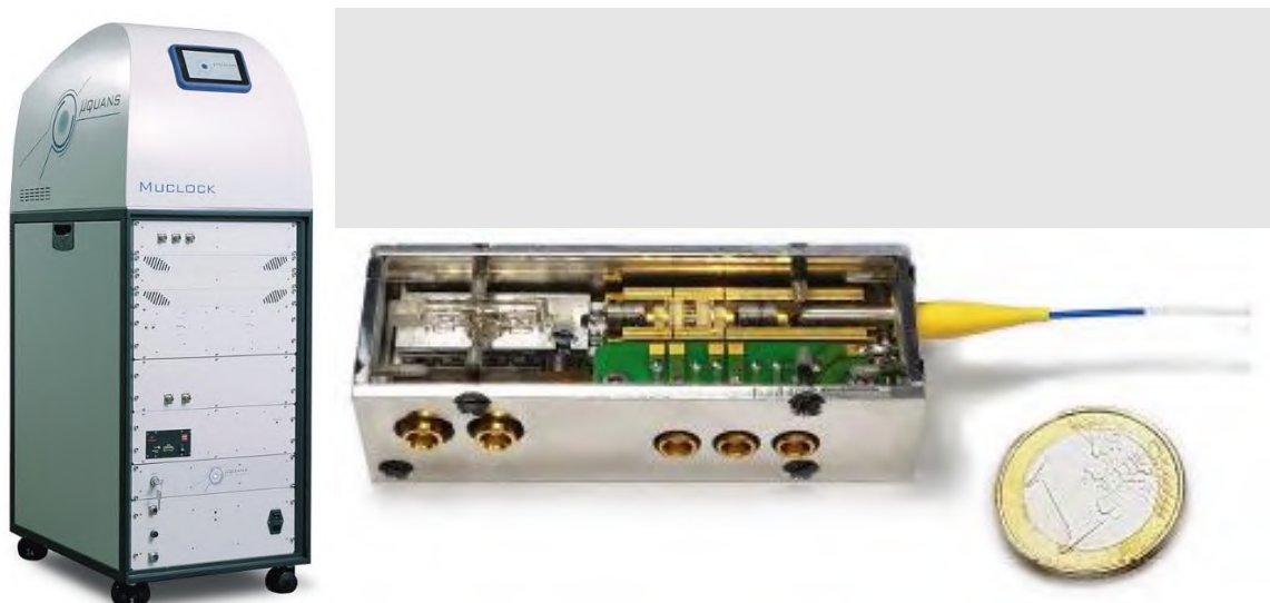
Figure 61 – A commercial cold-atom clock (left) and a prototype of an optical frequency standard based on two-photon transition in Rb (right). Note that in the latter the frequency comb necessary to translate the optical stabilised frequency into a microwave signal is not included [Strangfeld 2021]
