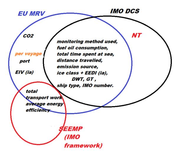
Explanatory Figure: per voyage (indicated in orange) is not a reporting obligation under the EU MRV Regulation but rather a monitoring obligation. Also, the SEEMP (MARPOL) is not reported, but contains energy efficiency parameters that should be available on a ship. Abbreviation: NT: net tonnage; DWT: deadweight tonnage; GT: gross tonnage; EEDI: energy efficiency design index; EIV: estimated index value.
