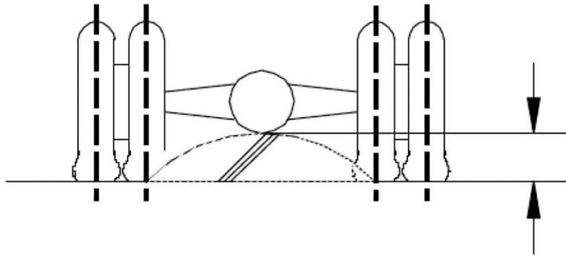
4.2.2. Where appropriate, the measurement of ground clearance shall be conducted on each of the several axles of a group of axles.
